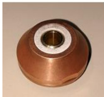
Figure 10: Top Detail appearance of the touch nozzle after 7 hours of cut
